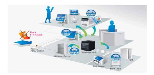
Figure 1 - Synology Disk Station Deployment
