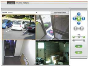
Surveillance Station 5 offers viewing of multiple cameras at once, remote pan/tilt/zoom control, remote access, motion detection, and audio recording. It is possible to schedule surveillance and recording to avoid wasting storage.
